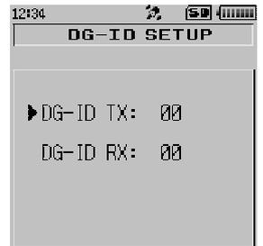
2. Press the **[GM]** key, then rotate the **DIAL** knob to set the transmit DG-ID number (DG-ID TX) to “50”.
